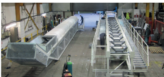
The main incline conveyor being manufactured at our works, ready for delivery.
