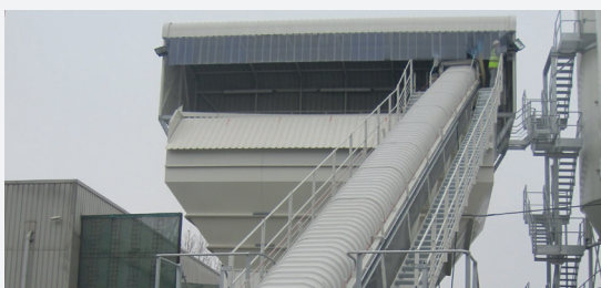
The completed conveyor fully installed and in production. It is capable of feeding the storage bins at 450 tonnes per hour.
